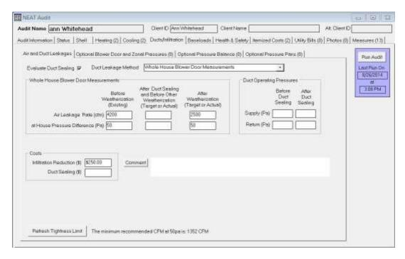
**(8) FOR MHEA ONLY**: there is a fourth option for **Duct Leakage Method**. This is the method of choice for MHEA audits. It is called **Pressure Pan Measurements.** Instead of a target blower door for after duct sealing, it asks for a sum of all pressure pan readings in the home. The target is typically the number of registers in the home, as we aim for 1.0 Pa per register (or less). However, it is important to have an
