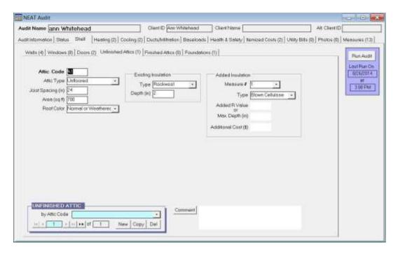
\*Note: Max Depth MUST be used for any attic surface that is limited by the depth of the joist/rafter such as a floored attic. In these cases, enter the thickness of the wood (e.g.: 2x8 floor joist – enter 8")
