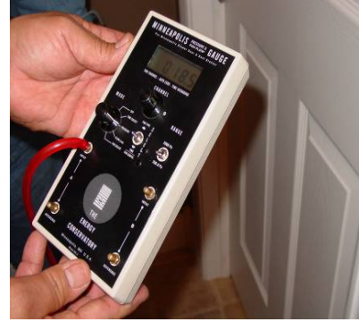
Figure 1152-1: Duct induced room pressure is 18.5 Pa!
