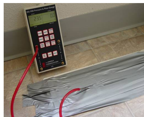
Figure 1141-2: Supply air register sealed with duct tape – note pressure pan reading of 23.5 Pa.
