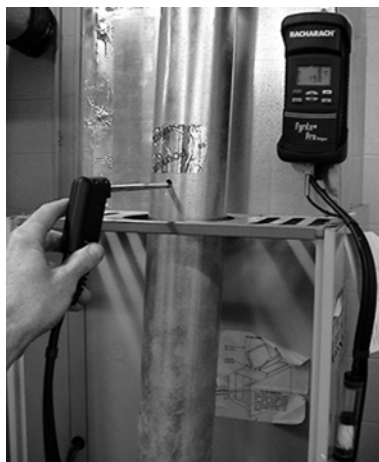
80+ Furnace: Measure draft and sample flue gases in the vent connector above the furnace. Only a licensed heating technician can perform this test. auditors may not do this process.
