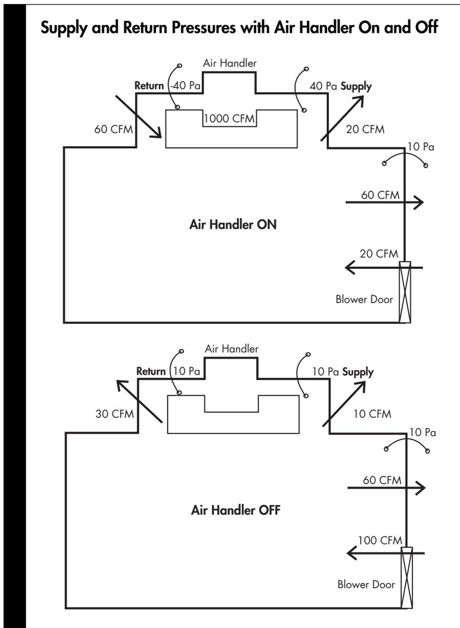
**Figure 1.** When the air handler is on, the pressures are increased across the supply leaks, leading to increased flow out of the supply leaks. The return section is at a lower pressure than the duct surroundings (and the house). The flow through the blower door that is required during a test to maintain the same envelope flow and pressure difference is then reduced from 100 CFM to 20 CFM. This change in flow at the same envelope pressure is the "DeltaQ".
