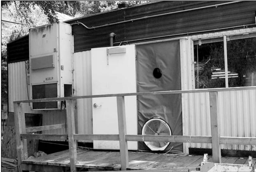
This building at LBNL was used to bench test the DeltaQ method. Taking the difference between flows at the blower door with the air handler on and off cancels out the building envelope leakage, leaving information about the duct leaks only.
