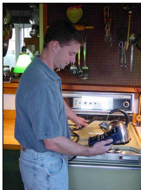
Testing gas oven for CO emission level
