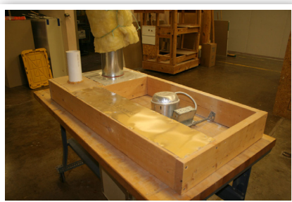
Cardboard and aluminum coil stock are fastened to openings. Students can work alone or in groups of two on this small prop.
