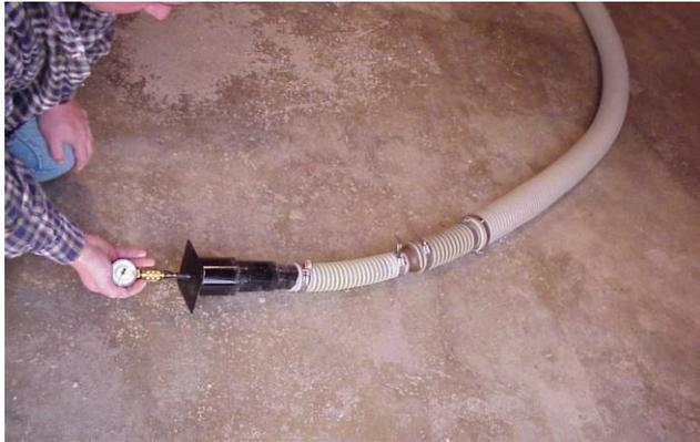
If the pressure is lower than the pressure at the outlet of the blowing machine, check the length of the hose for leaks. Continue to monitor the pressure while checking and sealing the hose.
