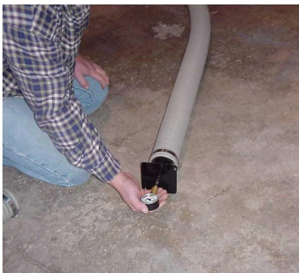
Test the hoses that you'll be using. The pressure at the end of the hose should be close to the same pressure reading you get at the blower. After the hose is extended, test the pressure at the end of the hose. It should be 3 to 4 psi.
