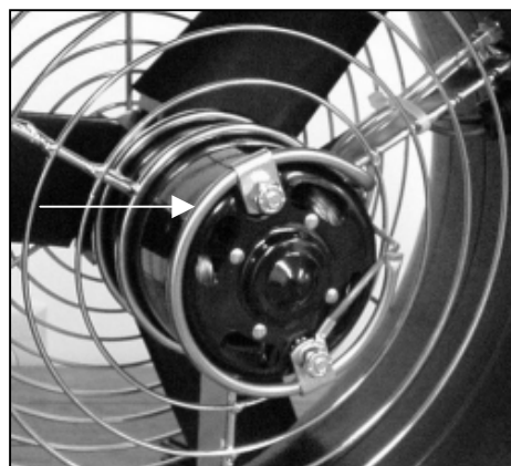
Flow Sensor on Duct Blaster Fan
