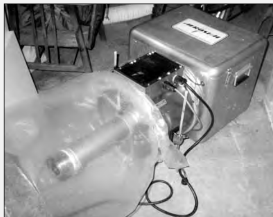
Figure A. Aerosol's injector consists of a blower, heater, and sprayer that are designed to create an air stream containing a mixture of water, sealant, and solvent. Plastic tubing connects the injector to the duct system.
