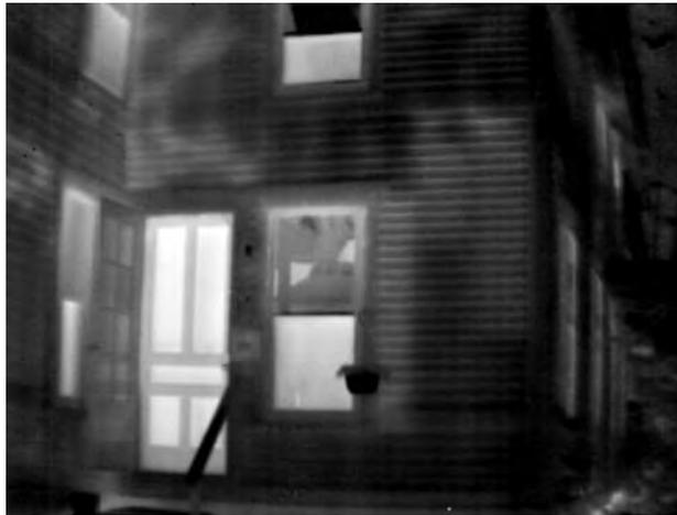
The quality of the images produced by modern IR systems is remarkable. Missing and poorly installed insulation is easily seen in this home.
