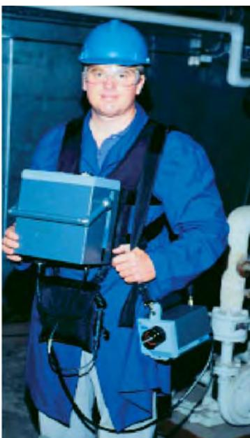
Author John Snell used a modern \$60,000, cryogenically-cooled, "portable" IR system in the early 1990s.
