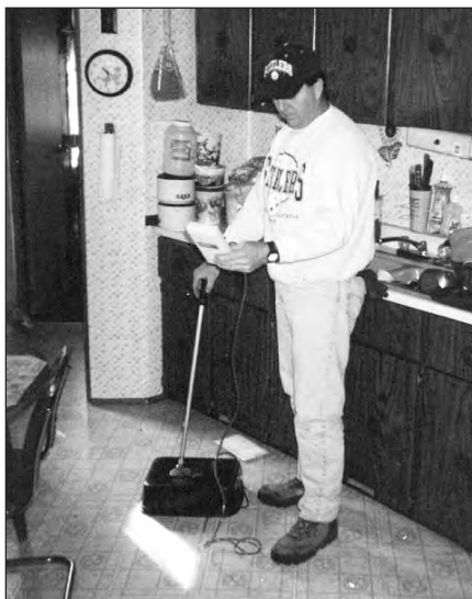
Along with a visual inspection, a pressure pan test is performed.
