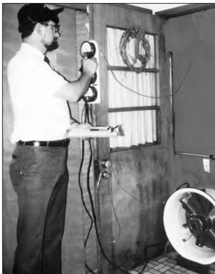
Rich Courtney, West Virginia Weatherization program specialist, takes a blower door reading in a mobile home to see how much air leakage there is. Rich has over 20 years' experience with retrofitting mobile homes and helped to develop a mobile home model used in statewide and national trainings.
