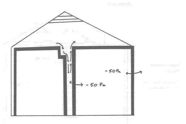
A story and a half house has interconnections between the basement, sidewalls and interior wall cavities to the first floor ceiling joists, kneewall attics and the peak attic. The house uses a first floor ceiling joists as a return chase for the upstairs. We measure a 15 Pa pressure at a second floor return register (with a pressure pan) 20 Pa pressure between the house and an interior wall cavity. What are the implications?
