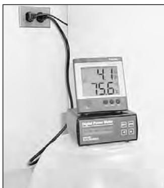
The "plug-and-play" Brand 4-1850WX watt-hour meter (bottom) and a Taylor multi-channel thermometer determine the fate of Michigan refrigerators during pre-inspection (in two hours).
