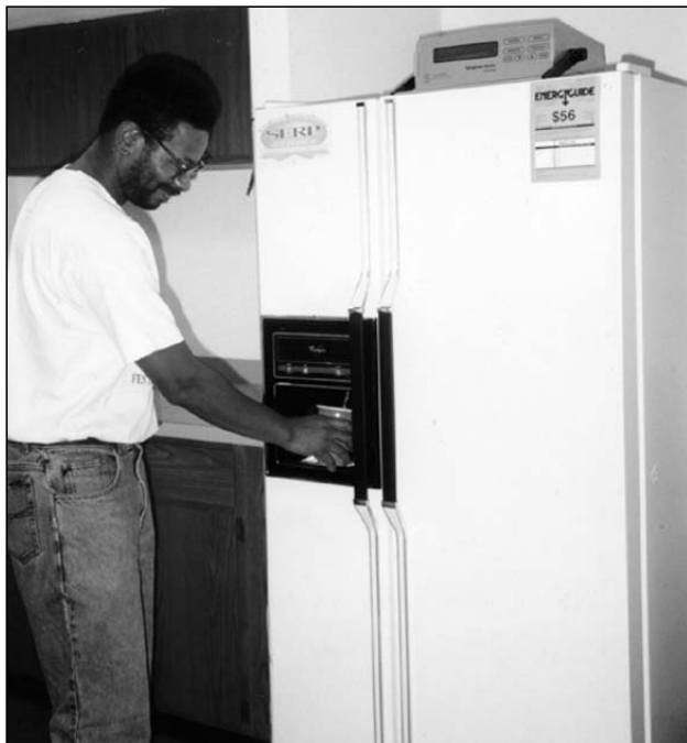
Monitoring the SERP refrigerator manufactured by Whirlpool. This unit auto defrosts via a series of very short-term defrost periods rather than one long one, which is the routine with most other household refrigerators.
