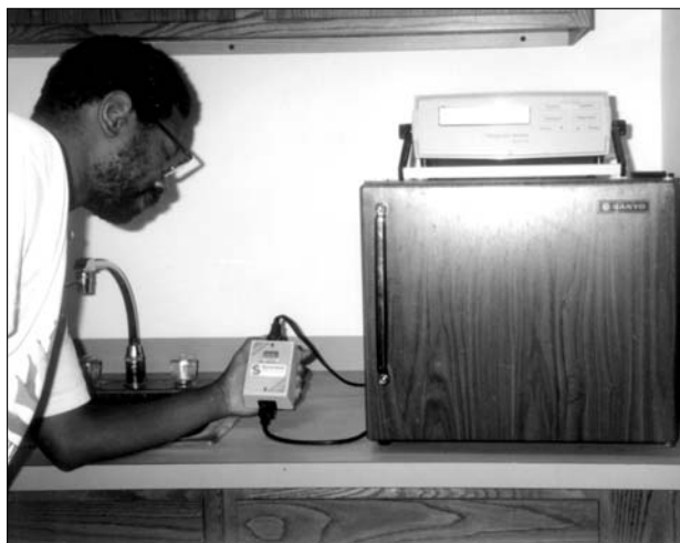
Glen Lewis, a researcher with the Synertech Systems Corporation, monitors the performance of a small refrigerator of the kind found in many dorm rooms. Such units are poorly insulated and appallingly inefficient (this one uses almost 200 kWh/year).
