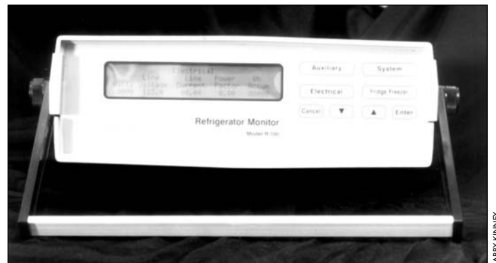
This R-100 data logger was designed to monitor the performance of refrigerators. It tracks 11 parameters and writes a time series data record at the interval chosen by the user, from one to sixty minutes. Its memory records over 15,000 data records before the newest data begins to overwrite the oldest.
