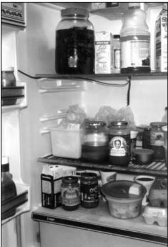
Combination temperature/light probe installed in a refrigerator's fresh food compartment. The time for setting up and verifying functioning of the instrumentation averages 15 minutes; data download and equipment stowage aver-
