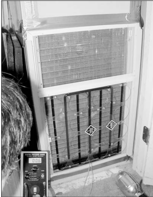
This Flow Meter is installed in a manufactured home heat pump. Tubes coming from the two manifolds allow for pressure measurements.
