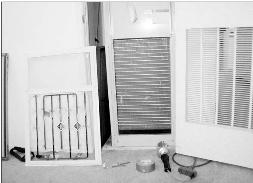
The Flow Meter has a spacer to fit most filter slots. This one fits in a 20 inch x 30 inch filter slot in a manufactured home.
