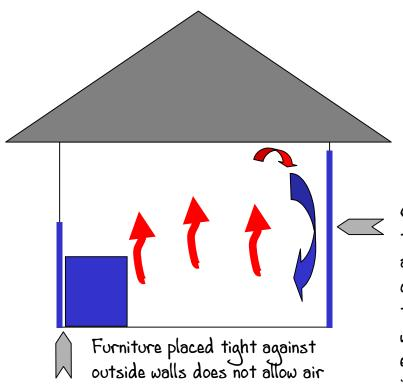
Furniture placed tight against outside walls does not allow air flow, creates a cool, high relative humidity area for moisture to condense, often resulting in mold growth.
