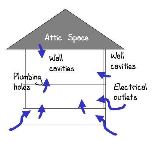
Air moves through holes, cracks and other penetrations within your home. The forces of wind, mechanical ventilation, & stack effect pull and push air around.
