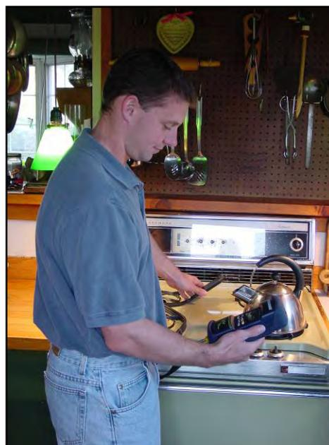
Testing gas oven for CO emission level
